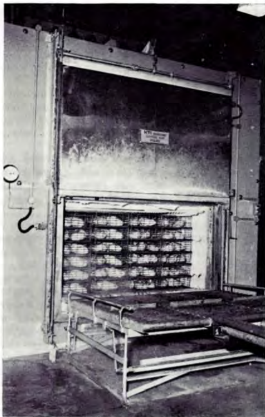
Above: One of the three blast freezers which together deal with about 35,000 chickens a day. Below: Insulator container vehicles being loaded—by electric fork lift trucks—with chickens from the cold store.
